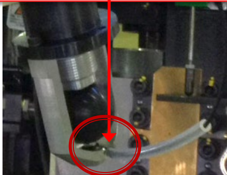
Bad: Silicone covers screw connector at sensor.
