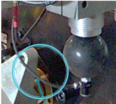
Good: free movement of sensor cable
