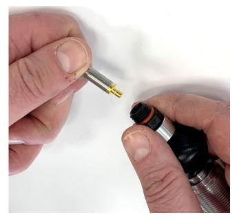
plug the microphone 4958 back into the MP21 connector.
