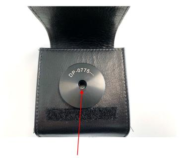
2. Disassembled - use the ¼" adapter for calibration.
