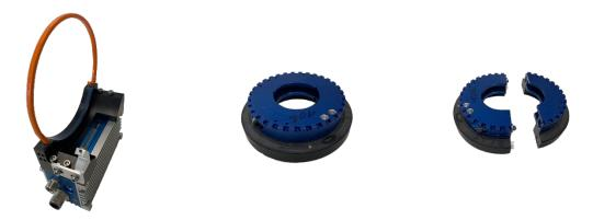
To achieve good measuring results, the TAC Sensor should be installed as close as possible to the test object. The mechanical coupling of the Rotor should be as direct as possible to the test object. A flexible coupling or a heavy shaft between the test object and the TAC Rotor will dampen the measurement signal significantly.
