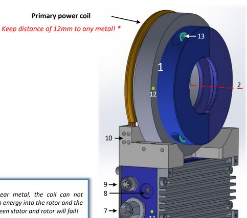
\* If mounted near metal, the coil can not transport enough energy into the rotor and the connection between stator and rotor will fail!
