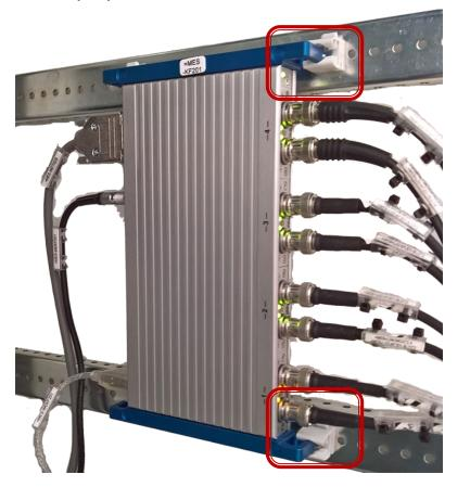
If placed horizontally, the rubber feet of the Tas box will provide isolation.
